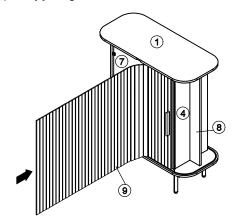
STEP 14 - Insert panel (9) along the slot.
