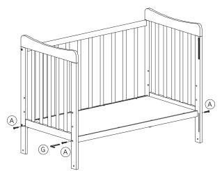
Note: To allow the fitting of the Drop Side Panel do not tighten fully at this stage
