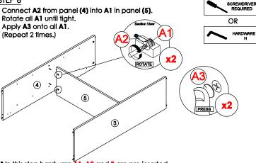
\* In this step hardware 1, A2 and B are pre-inserted.
