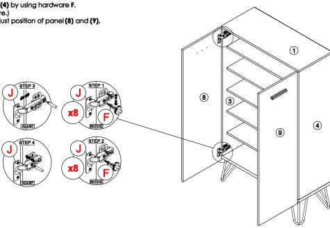
\* In this step hardware J have been assembled in panel (8) and (9).
