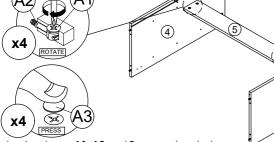
\* In this step hardware A1, A2 and B are pre-inserted.
