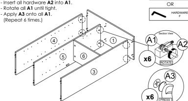
\* In this step hardware A1, A2 and B are pre-inserted.
