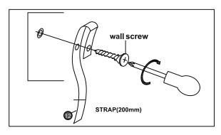
NOTE: Wall fixing are not supplied with this product as different wall materials require different types of fixing devices (such as Rawl plugs on brick work). You must use fixing devices suitable for the type of wall you intend to mount this product to. Please ensure that the head of any screw used has a diameter greater that the diameter of the mounting hole on the product and that the fixing is safe and secure before use.
