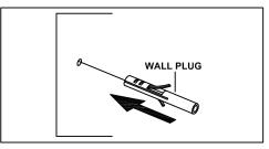
**STEP 3:** Pull the screw in the wall plug hole
