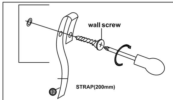
**NOTE :** Wall fixing are not supplied with this product as different wall materials require different types of fixing devices (such as Rawl plugs on brick work). You must use fixing devices suitable for the type of wall you intend to mount this product to. Please ensure that the head of any screw used has a diameter greater than the diameter of the mounting hole on the product and that the fixing is safe and secure before use.
