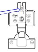
back and forth Loosen this screw, adjust by moving
