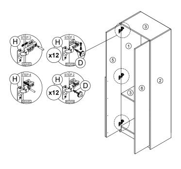
$<sup>^{*}</sup>$  In this step hardware **H** have been assembled in panel (5) and (6).
