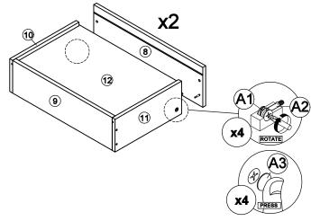
\* In this step hardware A1, A2 and B are pre-inserted.
