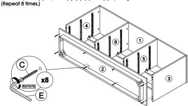
\* In this step hardware **B** are pre-inserted.
