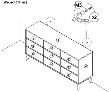
Assemble hardware M1 to M3 by using hardware M4. (Repeat 2 times.)
