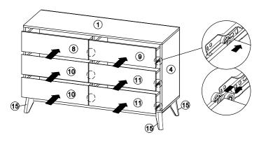
Third hole from the edge. Hole at the center. Third hole from the edge. \*Hardware L2 (L/R) shall be leaning against panel (8), (9), (10) and (11) when assembling.
