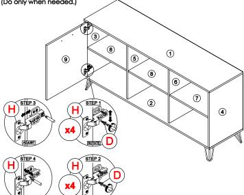
\* In this step hardware **H** have been assembled in panel (9).
