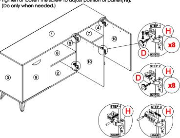
\* In this step hardware **H** have been assembled in panel (10).
