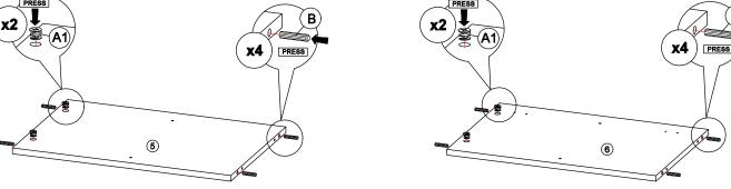
\* Ensure the arrows on hardware A1 point towards mounting positions.
