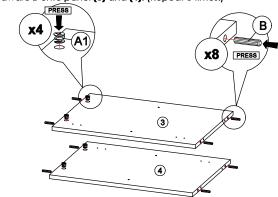
\* Ensure the arrows on hardware A1 point towards mounting positions.
