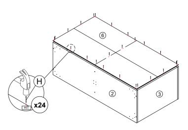
\* In this step hardware **B** are pre-inserted.
