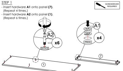
\* Ensure the arrows on hardware A1 point towards mounting positions.
