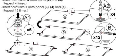
\* Ensure the arrows on hardware A1 point towards mounting positions.
