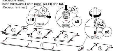
\* Ensure the arrows on hardware A1 point towards mounting positions.
