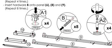
\* Ensure the arrows on hardware A1 point towards mounting positions.
