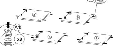
$\ensuremath{^*}$  Ensure the arrows on hardware  $\ensuremath{\mathbf{A1}}$  point towards mounting positions.
