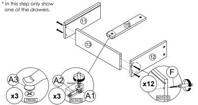
\* Ensure the arrows on hardware A1 point towards mounting positions.
