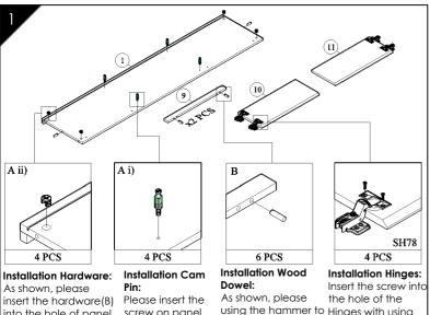
screw on panel into the hole of panel (1) using a (1).Make sure the arrow point out screwdriver.
