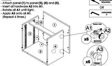
\* In this step hardware A1, A2 and B are pre-inserted.
