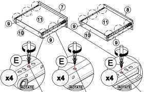
Third hole from the edge. Hole at the center. Third hole from the edge. \*Hardware L2 (L/R) shall be leaning against panel (7) and (8) when assembling.
