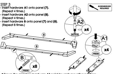
\* Ensure the arrows on hardware A1 point towards mounting positions. STEP 5
