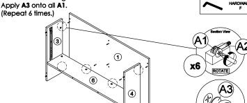
\* In this step hardware A1, A2 and B are pre-inserted.
