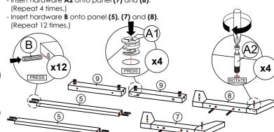
\* Ensure the arrows on hardware A1 point towards mounting positions.
