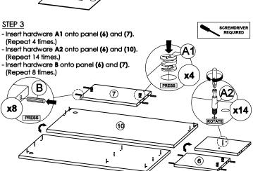
\* Ensure the arrows on hardware A1 point towards mounting positions.
