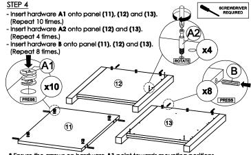
\* Ensure the arrows on hardware A1 point towards mounting positions.
