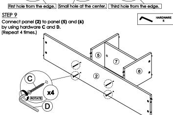
\* In this step hardware B are pre-inserted.
